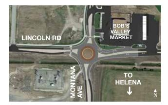
A single-lane roundabout with a westbound right-turn bypass lane will be constructed. The bypass lane will address the high amount of westbound to northbound right-turn movements during the evening rush hour.
