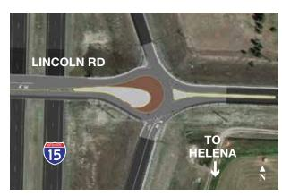
A single-lane roundabout with a northbound right-turn bypass lane will be constructed. The bypass lane will increase the capacity of the northbound off-ramp to reduce stacking on I-15.
