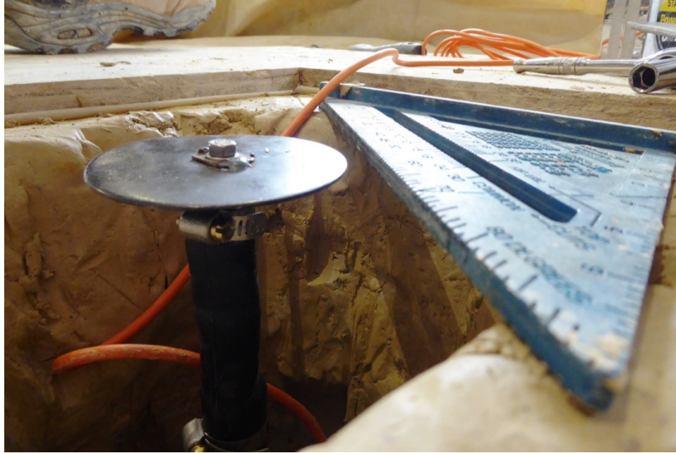
Figure 4-4: Position of the measurement point with respect to the subgrade surface.
