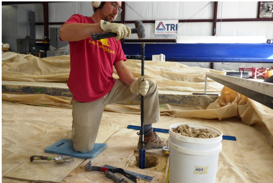
Figure 4-2: Installing LVDT anchor.
