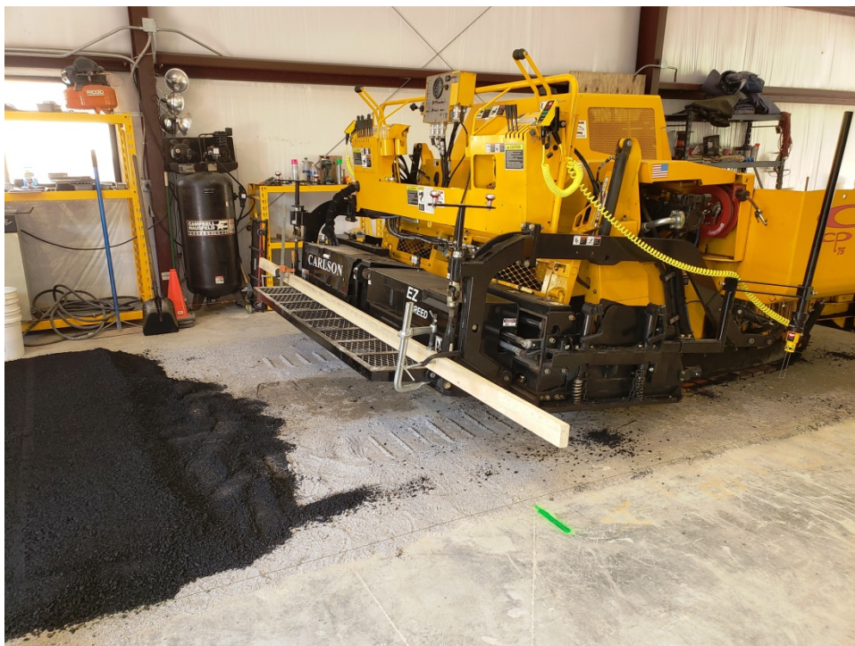
Figure 7-1: Placement of the hot-mix asphalt.
