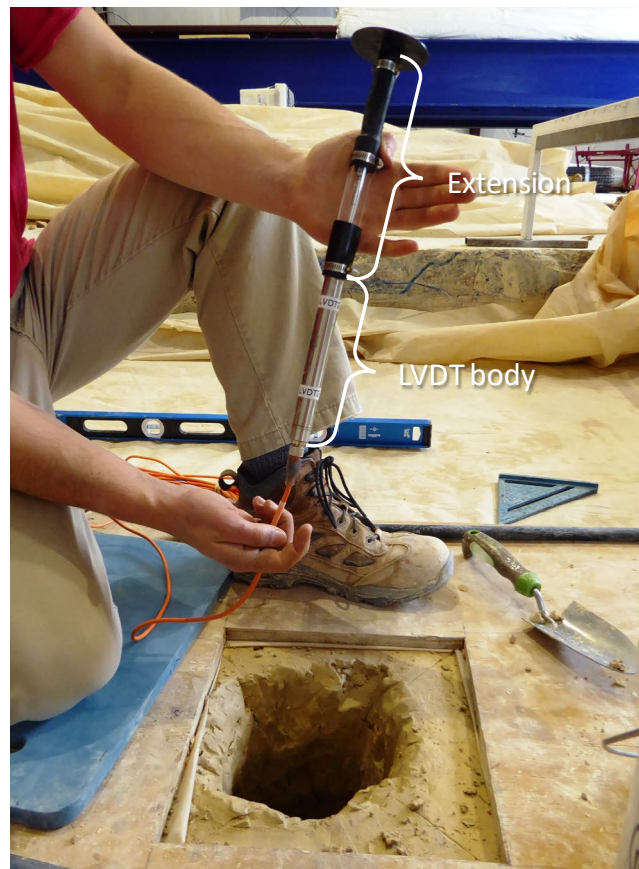
Figure 4-3: LVDT sensor prior to installation.
