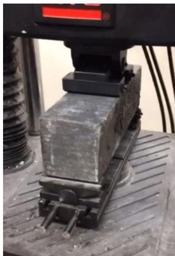
Figure 3: Example flexural test performed on an earlier MT-UHPC mix at MSU
