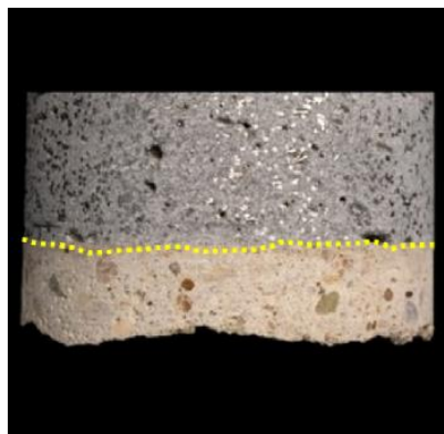
Figure 1: Example direct tension bond strength core specimen [10]
