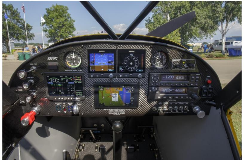
Aerotronics painstakingly designed, cut, and helped install the impressive, modern panel in the AOPA Sweepstakes Super Cub Photo by Mike Fizer
