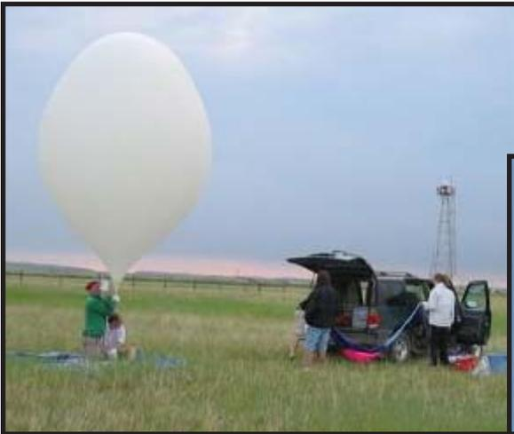
*Occasionally, the U of M Dept of Physics and Astronomy uses MDT's airport at Augusta for scientific balloon launches. Last month they released this balloon which carried new sophisticated temperature and humidity sensors along with A, B and C UV sensors to correlate data on ozone concentrations.*
