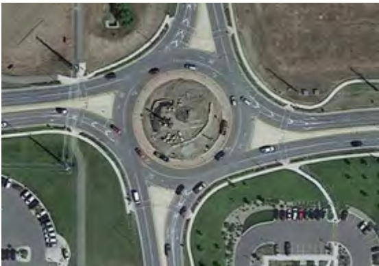
Figure 11.15: Multi-Lane Roundabout – King Avenue and 40th Street, Billings, MT
