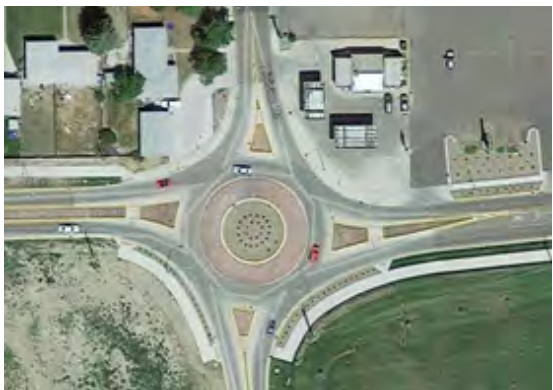
Figure 11.17: Single-lane Roundabout – Smelter Avenue and Division Road, Great Falls, MT
