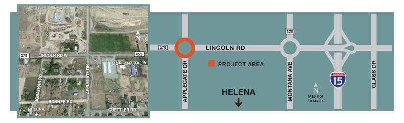
MDT evaluated several options for improving the intersection including traffic signals and a four-way stop. Based on statewide safety data, a traffic analysis, and input from the community, MDT determined that the intersection would benefit most from a roundabout design.
