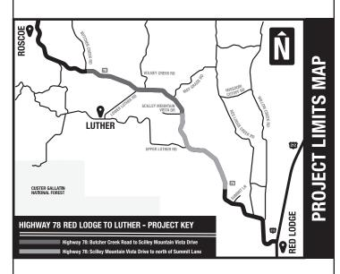
Roadway designs are being developed to reduce the roller coaster effect and increase sight distance. Hwy 78 shoulders will be widened to four feet on each side and pull out areas will be added. In total, nearly 11 miles of roadway will be improved.
