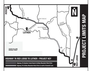
Roadway designs are being developed to reduce the roller coaster effect and increase sight distance. Hwy 78 shoulders will be widened to four feet on each side and pull out areas will be added. In total, nearly 11 miles of roadway will be improved.
