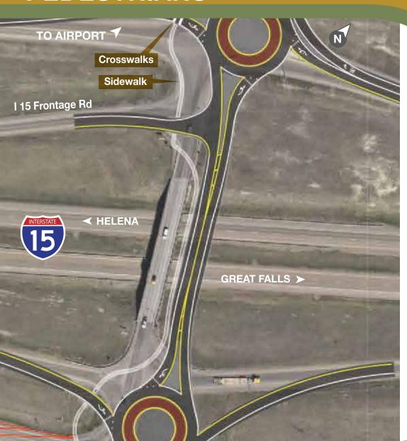
Sidewalk and crosswalks will provide safe passage over the overpass bridge and connectivity between the two roundabouts.
