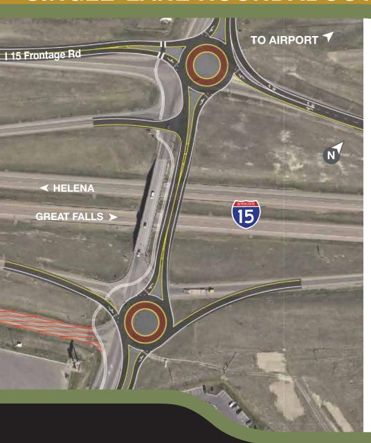
Two roundabouts are replacing the on- and off-ramp intersections. The current intersections are difficult for trucks or other commercial vehicles to navigate. This leads to reduced traffic flow.
