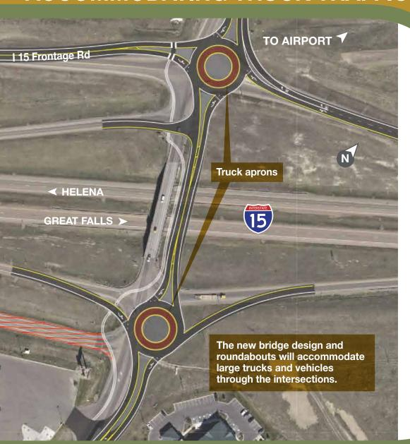
The new single-lane roundabouts will include truck aprons in the center of the roundabout.
