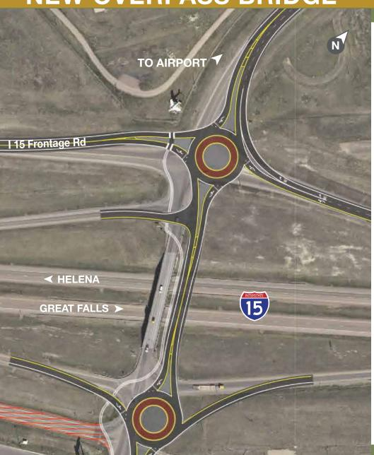
Based on input from the community, MDT decided to build a new interchange structure to the east of the current bridge, allowing the current overpass to continue to function during construction.
