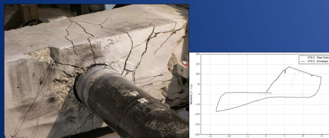
Example of test specimen VT2.5 with degraded concrete cap – Non-Ductile Behavior with pinched hysteresis response
