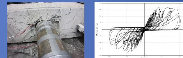
CT1 - oversized pile with significant cap deterioration
