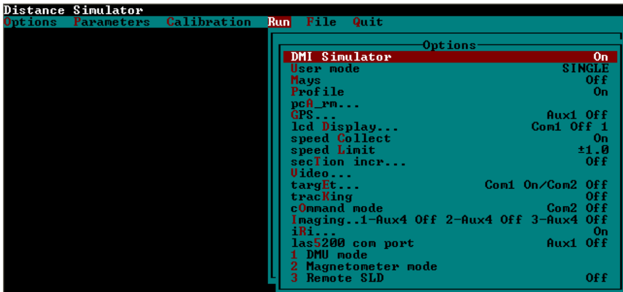
Figure 4-6. Run Options Menu Toggling Distance Simulator On for Pre-Run Bounce Test.
