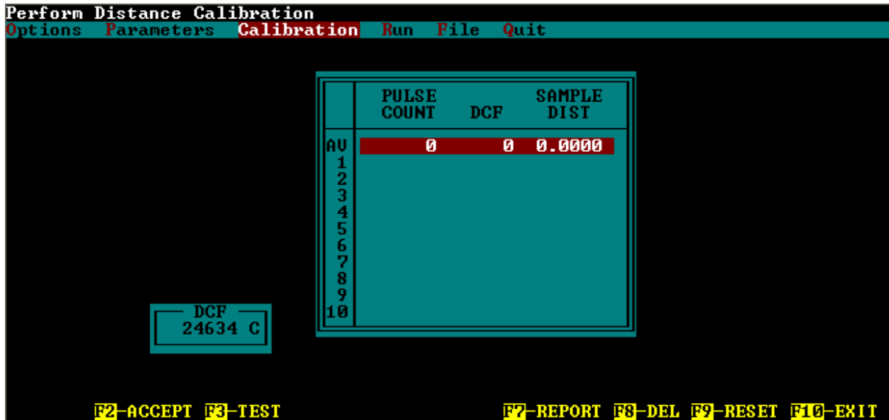
Figure 3-10. MDR Software Distance Calibration Screen Before Performing DMI Calibration.
