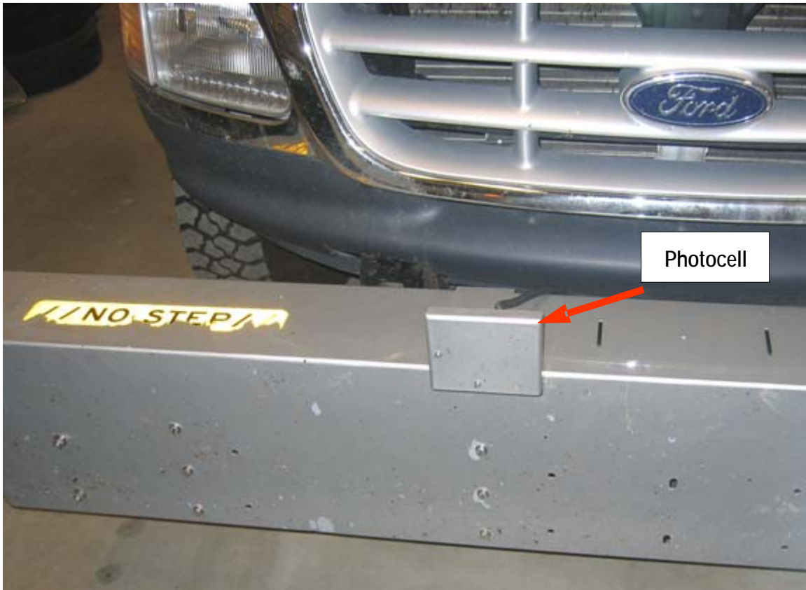
Figure 2-2. Photocell Mounted on Sensor Bar.
