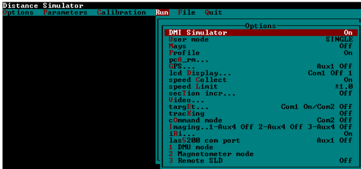
Figure 3-6. Run Options Menu Toggling Distance Simulator On.
