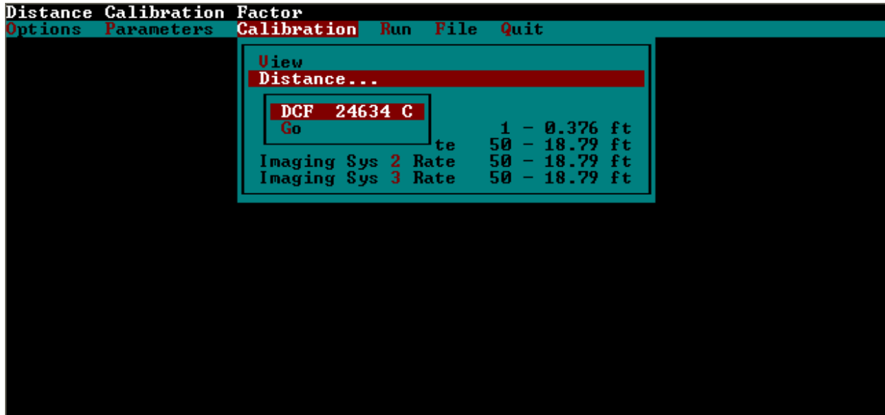
Figure 3-9. MDR Software Distance Calibration Menu.
