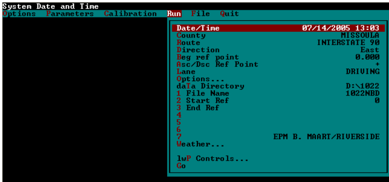
Figure 4-9. MDR Software Run Menu for Profiling.
