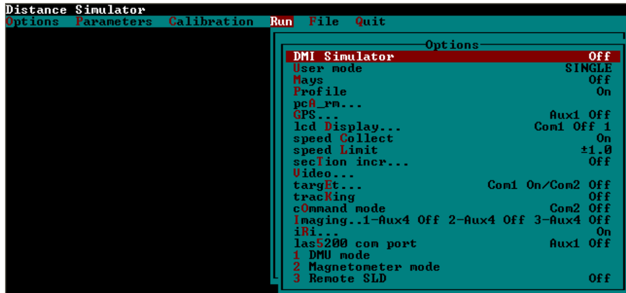
Figure 4-8. Run Options Menu Toggling Distance Simulator Off for Pre-Run Bounce Test.
