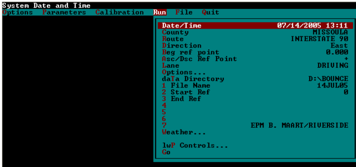
Figure 4-5. MDR Software Run Menu for Pre-Run Bounce Test.
