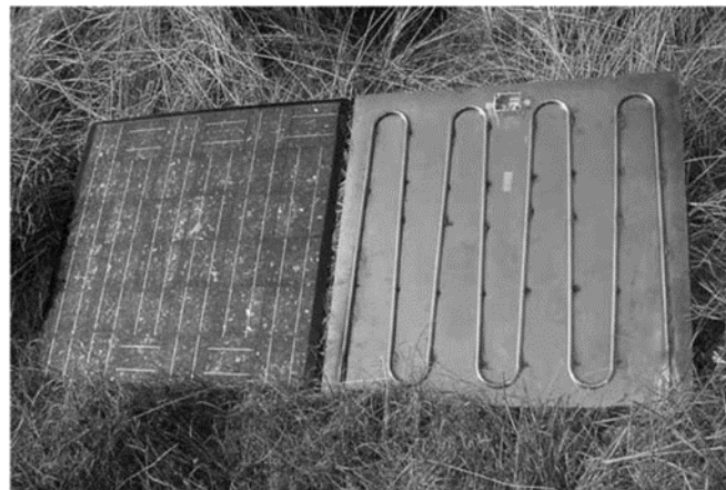
Figure 19. Front and back of a PVT panel (Bakker et al., 2005)
