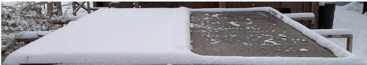
Figure 40. Photo of the deck model surface during the storm. Heat exchanger pipes have spacing of 30 cm and 20 cm in left-side and right-side model deck, respectively (Bowers Jr, 2016).
