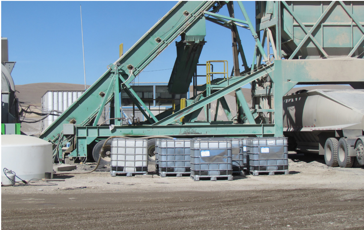
Figures 7 and 8- Evotherm additive baskets at mix plant facility
