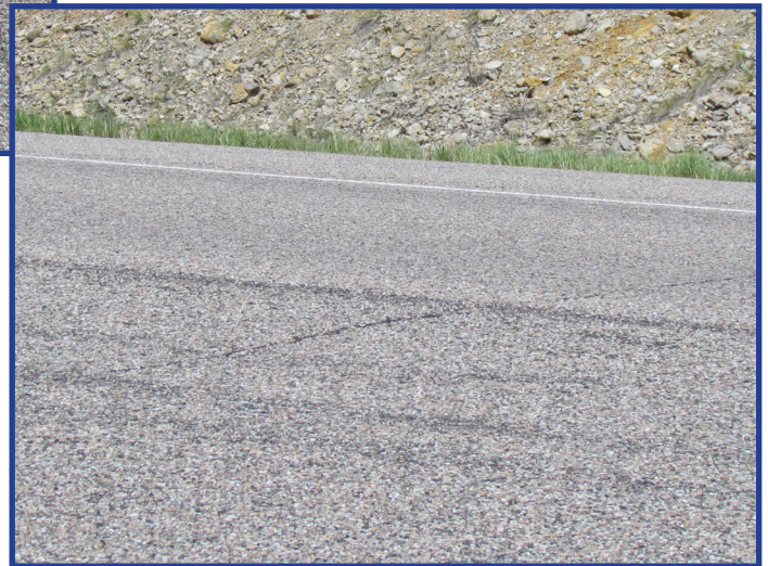
Figure 12- Examples of reflective cracking in warm mix asphalt pavement (top) and hot mix asphalt pavement in northbound lane (right)
