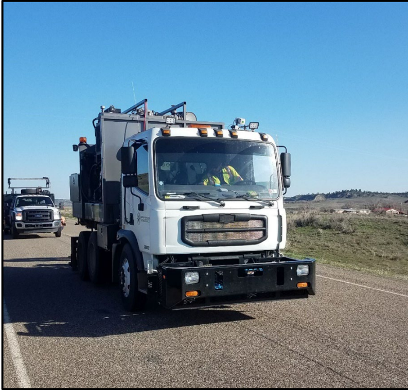
◀ Front view of the SPT Noiseprint Rumble Strip Mill truck used on the project.
