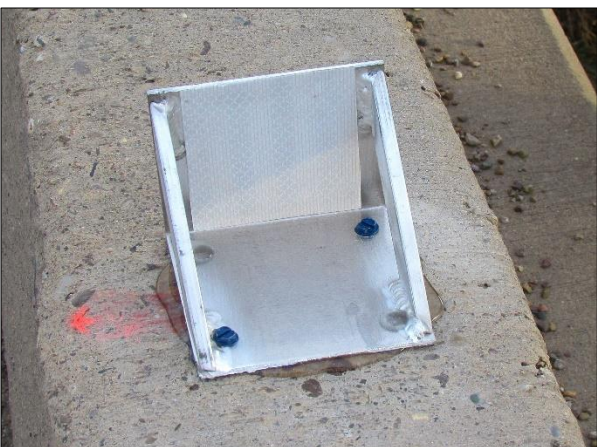
← Test Prototype Unit T3; glue and screw anchor attachment.
