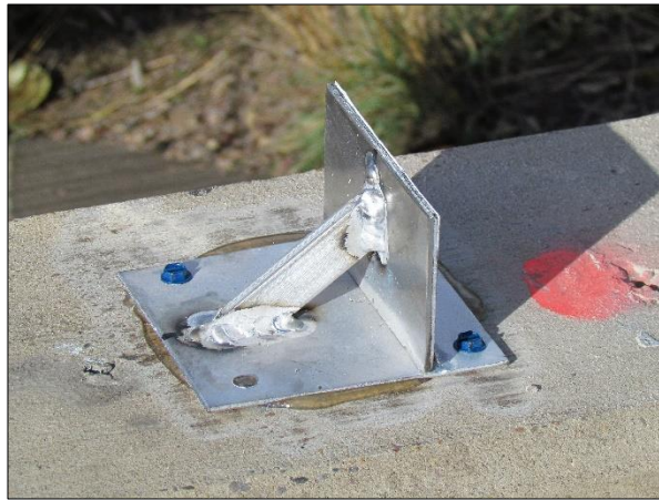
← Test Prototype Unit T4; glue and anchor attachment.
