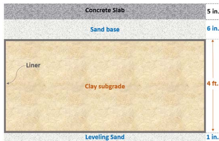
Figure 1. Schematic as-built cross-section of the MDT's original testing area (not to scale).
