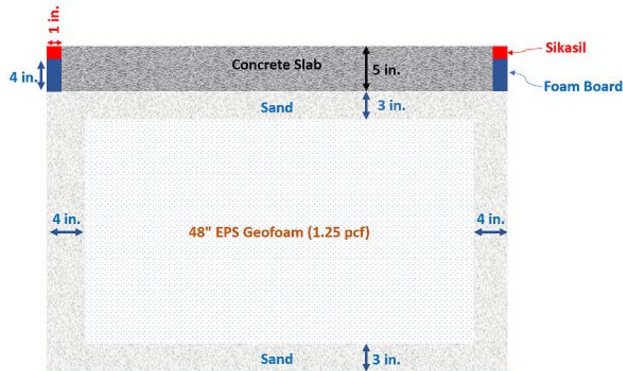
Figure 2. Schematic as-built cross-section of the MDT's preliminary alternative testing area (not to scale).
