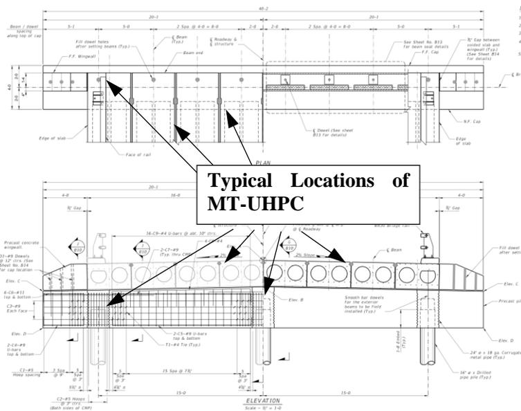
Figure 1: Trail Creek Bridge Structural Drawings
