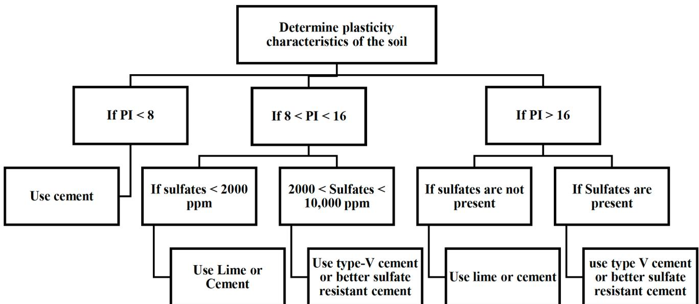
Figure 1: Flowchart to select optimal additive type for chemical in Montana.
