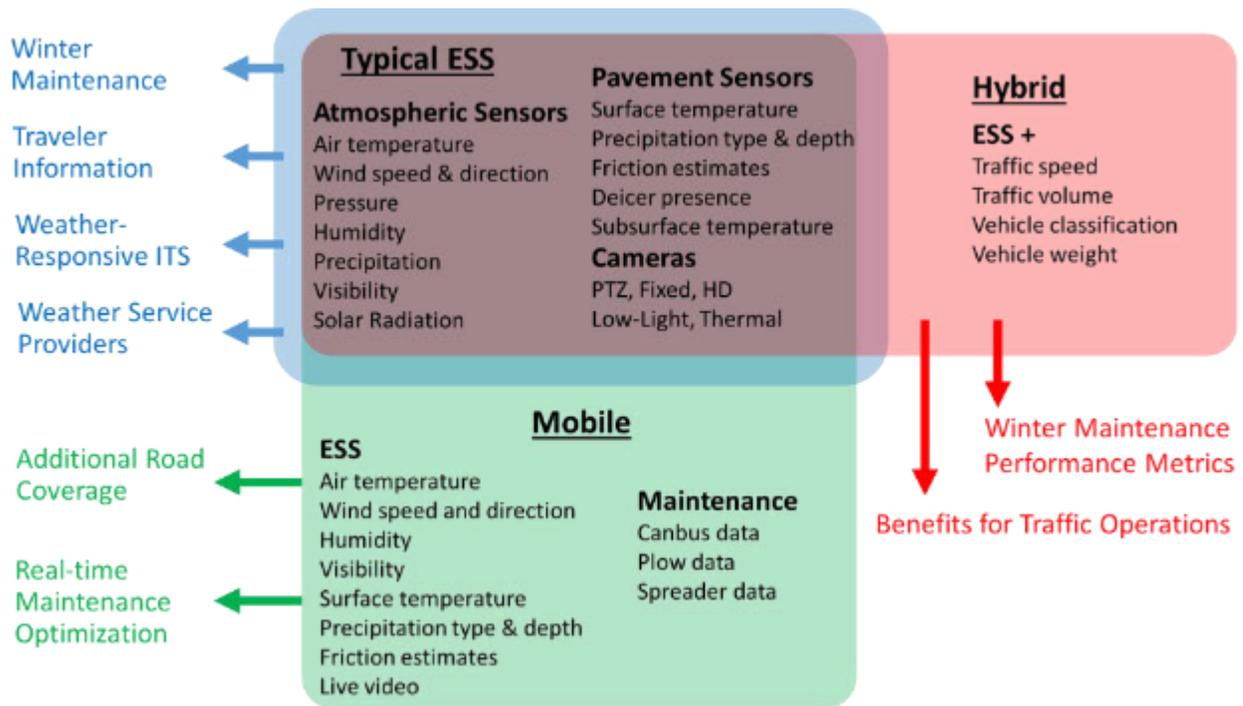
Figure 1: RWIS Components and Uses
