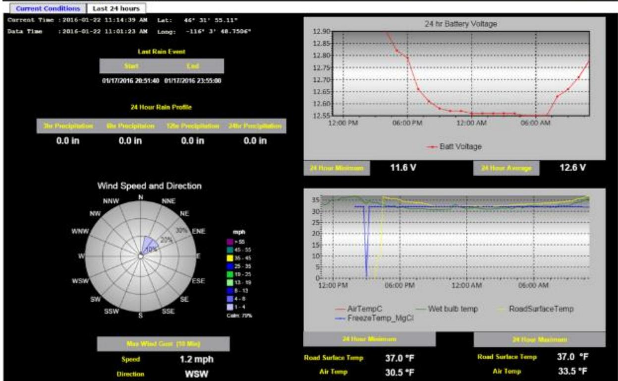
Figure 42: RTMC Pro Software Example (gc.clearwatercounty.org)
