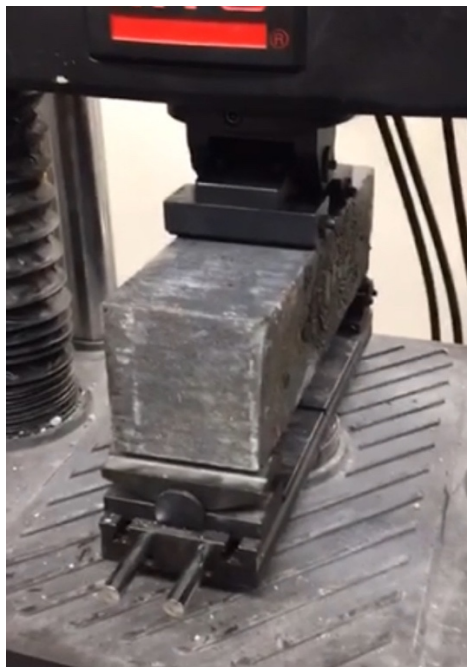
Figure 6: Flexural test specimen in load frame
