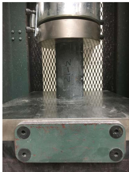
Figure 5: Compression cylinder in load frame
