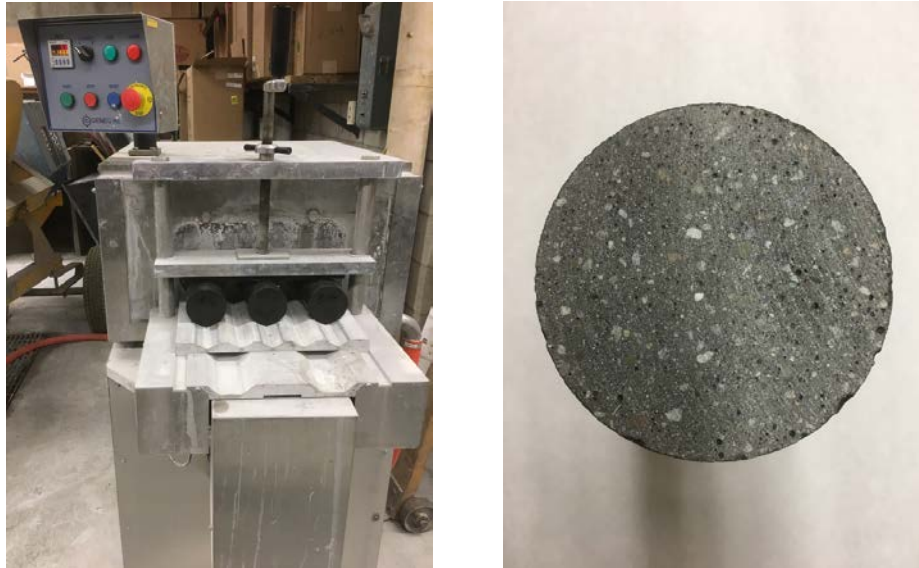
Figure 4: Cylinder end grinder and prepared specimen
