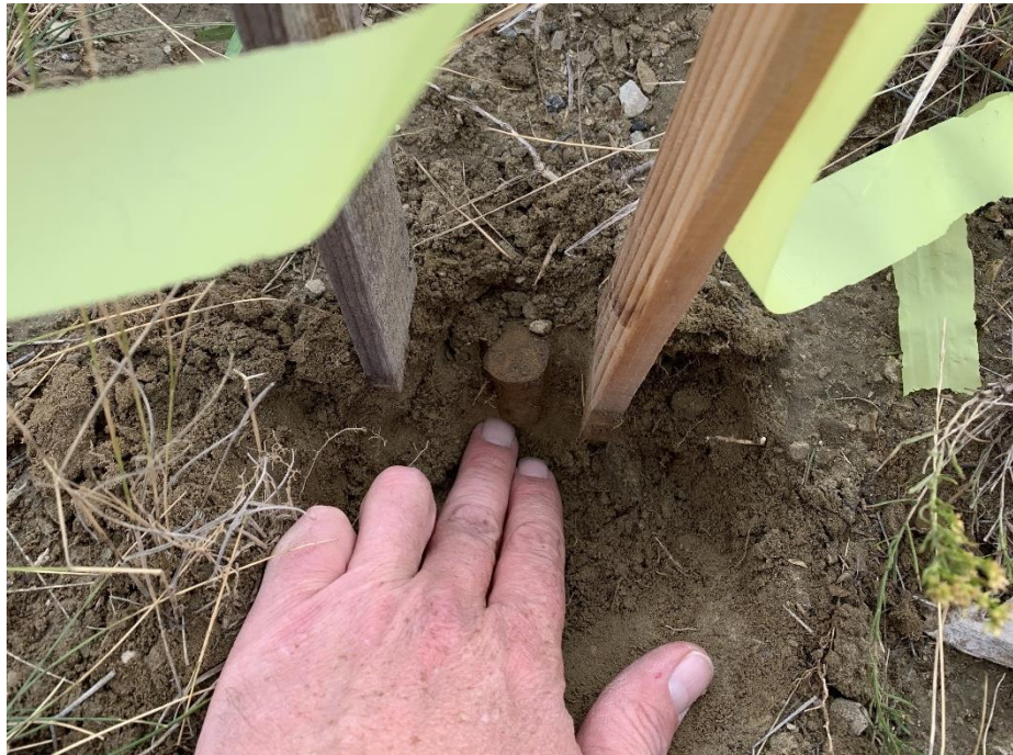
Figure 6-4: Right-of-way reference pin
