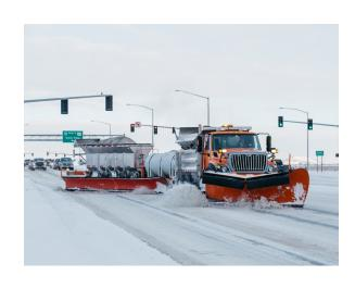
The Tow Plow is a steerable trailer-mounted plow that is pulled behind a plow truck. The Tow Plow can be rotated to one side of the truck, which doubles the plow width. The 26-foot-wide plow gives the operator the ability to move snow from two lanes of roadway in one pass.
