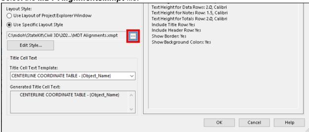
8. In the *Table Style* section, select *Use Specific Table Style* and click the ellipsis to navigate to the same folder as in Step 7. Select the *MDT Alignments.xmpa* file. Ensure the *Title Cell Text Template* is set to *{Object Name}*.
