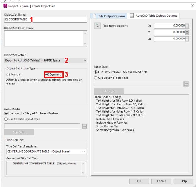
7. In the *Layout Style* section, select *Use Specific Layout Style* and click the ellipsis to navigate to the following folder:
