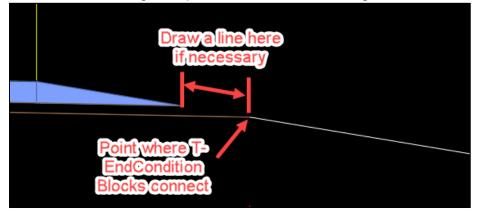
Additionally, the "VARIES" text in the *T-EndCondition* blocks may need to be changed to "EXISTING" or "AS CONSTRUCTED."
