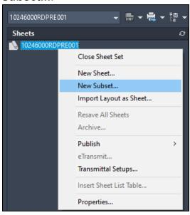
2. Type "**ROAD PLANS**" for the Subset Name as and select **OK** in the Subset Properties dialog to create the subset.
