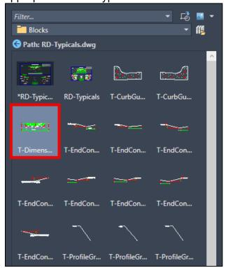
**NOTE:** The *T-EndCondition* blocks are set up to connect to the edge of the CAC on the inslope, so a line or polyline may need to be drawn to connect the rest of the surfacing inslope, like shown in the image below:
