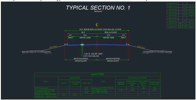
Example of a plotted typical section:
