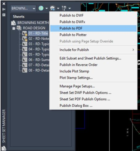
2. Select an appropriate location to save the PDF then select *Print*. A processing window will appear to display progress. Once the print job is complete, the following message will display on the status bar on the bottom right side of the application window, like shown in the image below:
