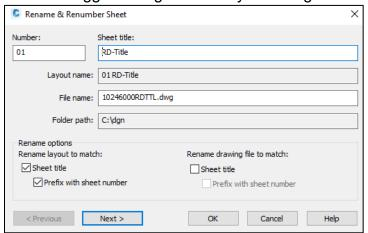
**NOTE:** The process of renaming and renumbering the sheet through the SSM will automatically populate sheet numbers on the layouts like shown below.
