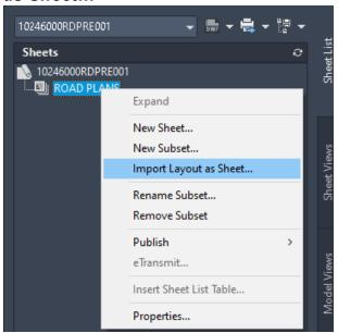
2. In the *Import Layouts as Sheets* dialog, select *Browse for Drawings...*. Browse to the project's RD folder on Autodesk Docs. Using shift or control, select all the drawings containing the desired layouts for plotting and select *Open*.
