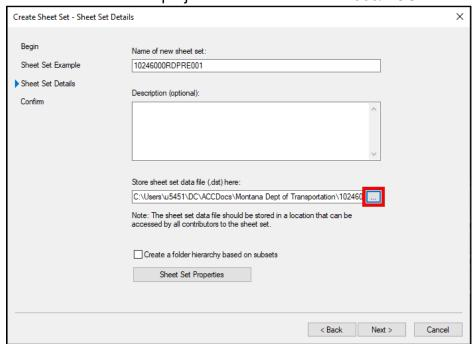
6. Click the Sheet Set Properties button and populate the custom properties with the appropriate project information in the Project Control and Sheet Set Custom Properties sections. Type %% to blank out a field, such as the reviewed and checked names and dates, until it is ready to be populated later. Setting the properties will automatically populate all title blocks with the project information when layouts are added to the sheet set.
