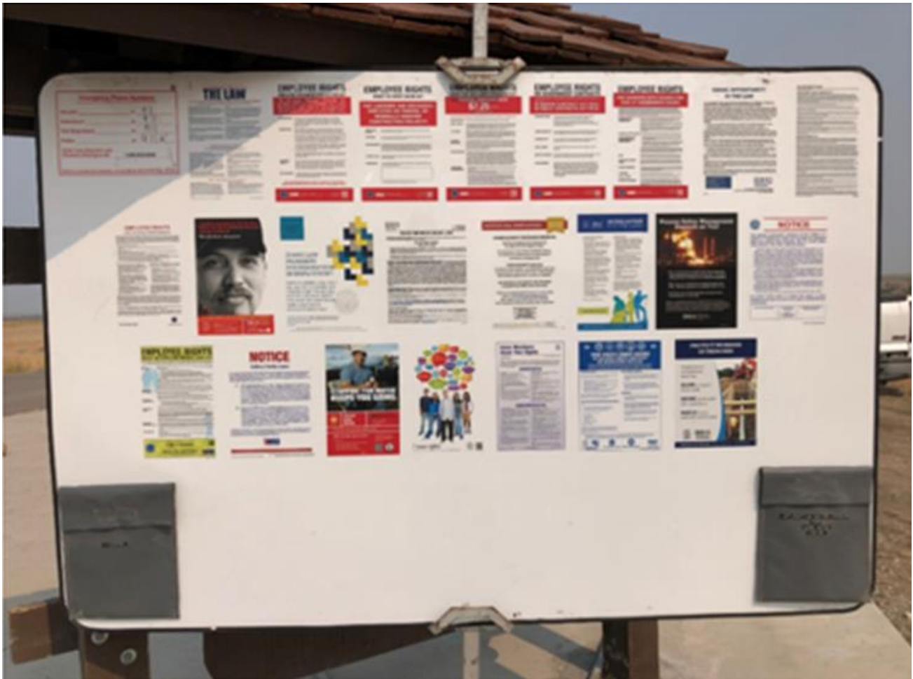
Required notices and posters are affixed to a white board, which is held by a wind jammer. Contract specific documents are in the weatherproof pockets.
