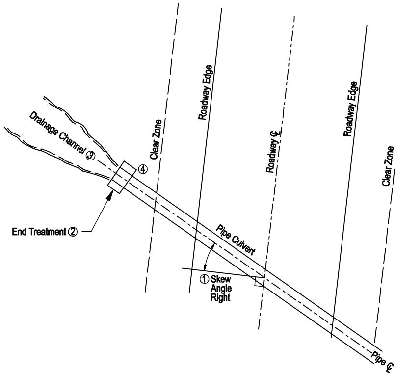
① A skew angle right is one where the pipe centerline is to the right of a line extended perpendicular from the roadway centerline. A skew angle left is one where the pipe centerline is to the left of a line extended perpendicular from the roadway centerline.
