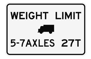
The new posting on the MT 200 Buffalo Spring Creek Bridge applies to SHVs; it limits the maximum gross vehicle weight of single-unit vehicles with 5, 6, or 7 axles to 27 tons.
