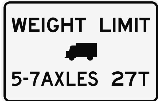
The new posting on the Dry Wash Bridge applies to SHVs; it limits the maximum gross vehicle weight of single-unit vehicles with 5, 6, or 7 axles to 27 tons.
