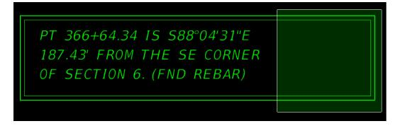
If you would like to resize the cell place a fence as shown above. Within the fence dialog box select Manipulate Fence Contents and from the box that pops up select stretch cells.
