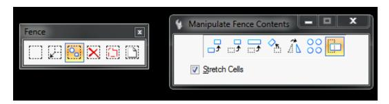
Move the fence and the section tie cell border will adjust.
