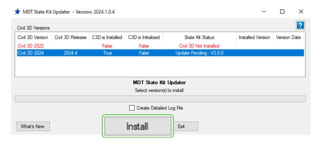
During State Kit installation, Storm and Sanitary Analysis software may be launched if not previously initialized. It will launch, remain open for a moment, and close on it's own.
