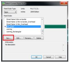
Enter the new panel style name to be for example **test\_blue** and click ok:
