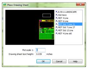
This scale is used because the 25 sheet format uses this feature for referencing in the 25 sign designs from the <u>sign working areas</u> to the <u>sign sheet frames</u>, and the many sign sizes which would be necessary to fit the sheets for standard printing. Reference the Sign Design in the Sign Working Area to the Sign Sheet Frame (Working Area). This way changes can be made in the future. If you scale the sign design to the Calc Sheet, you will have to start over to modify the sign design.
