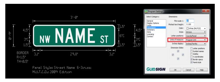
If in Program Settings -> Dimensions I then change Units of Measure to be Sub Unit, and I then click on Place Dimensions again, then as you can see my sign is dimensioned in inches in this case and I can see 2 decimal places.
