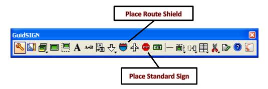
The <u>Place Standard Sign</u> icon is used for placing typical signs in your plan sheets or layouts. These cells will not place within a Sign Panel and is not recognized as panel objects.
