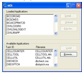
Under the Utilities/MDL Applications, click on the browse button of the MDL box and choose the gs8i.ma file. **GuideSIGN** will now load. You can close the MDL box now and proceed designing signs.
