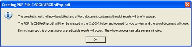
11. The 8½X11 pavement preservation plan sheets will be plotted to plot files. Microsoft Word will then open and the plot files will be inserted into a blank Word document. The Word document will then be saved and the PDF will be created by printing the Word document to the PDF995 printer installed on the user's computer. Once the PDF file has been created, Microsoft Word will close and the Word document will be deleted.
