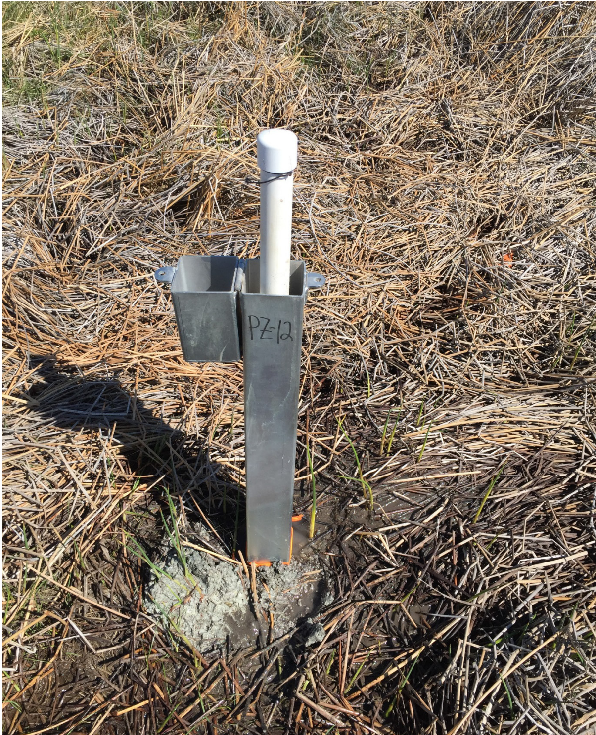
Photograph 4. PZ-12 Outer Steel Casing Settled into Ground
