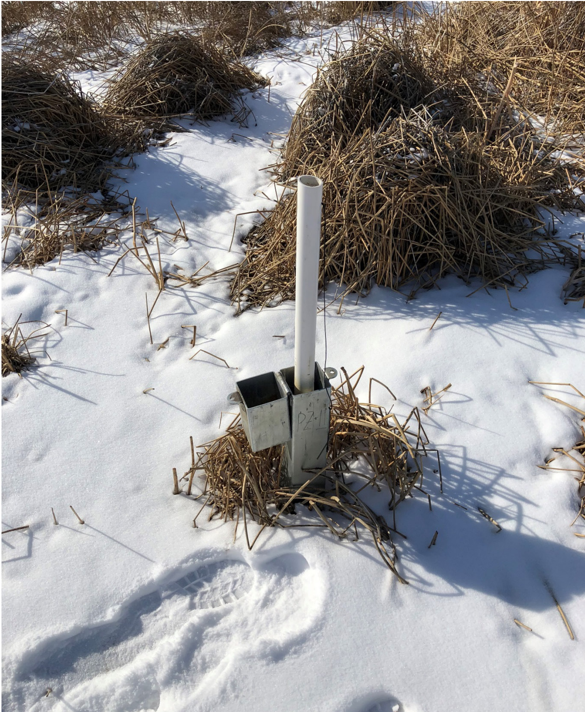
Photograph 3. PZ-11 Outer Steel Casing Settled into Ground
