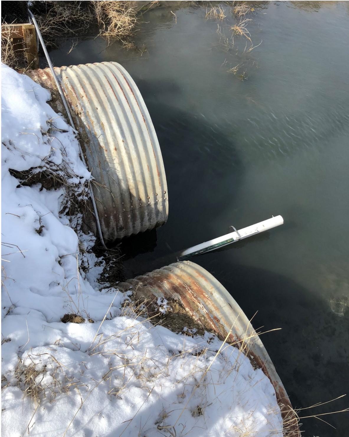
Photograph 5. Stilling Well SW-02 Damaged by Cattle
