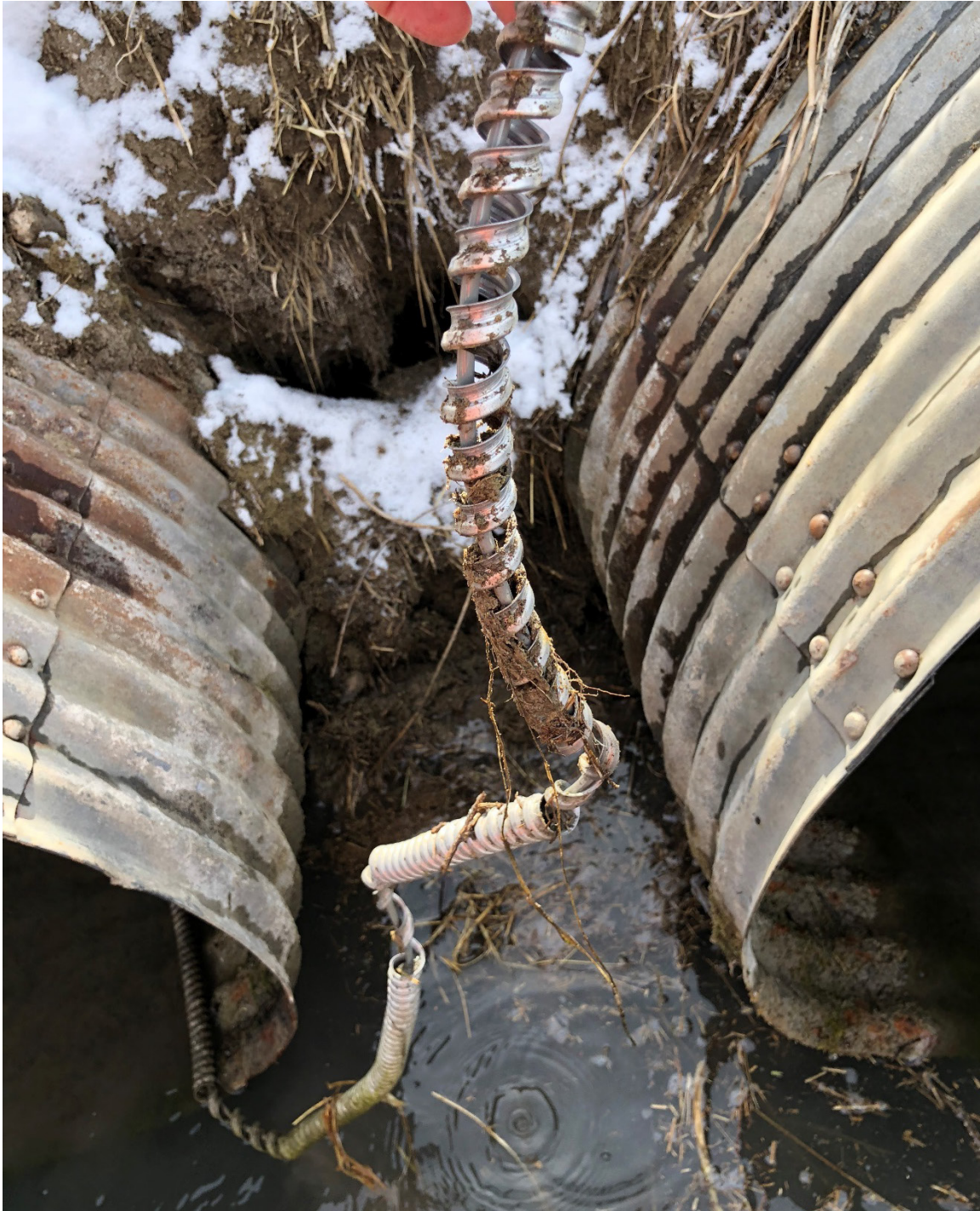
Photograph 6. SonTek-IQ Pipe Cable Damaged by Cattle
