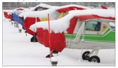
**Don't forget a thorough preflight**. It may have been a while since you've last flown, so now's an important time to complete a full preflight inspection. Check everything as if you are demonstrating for an examiner. Remember that tires may lose pressure when the temperature drops; all frost or snow needs to be removed; and small animals want out of the cold too, so they may have made a home in an engine cowling.
