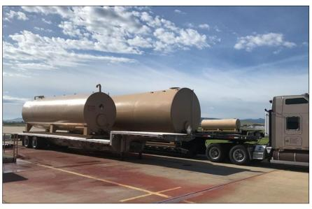
10,000-gallon tank on the left is replaced by the 25,000-gallon tank on the right Photo credit: Helena Independent Record
