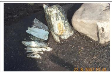
Anthophyllite asbestos ore encountered during excavation activities within the City of Bozeman. Asbestos fragments and shards may also be present in excavations.
