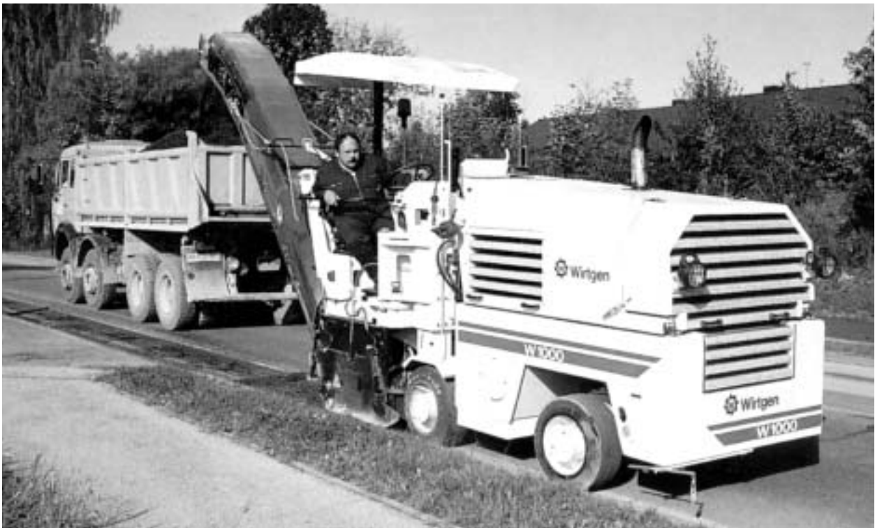
Figure 8-8: Small self loading, partial lane width milling machine
