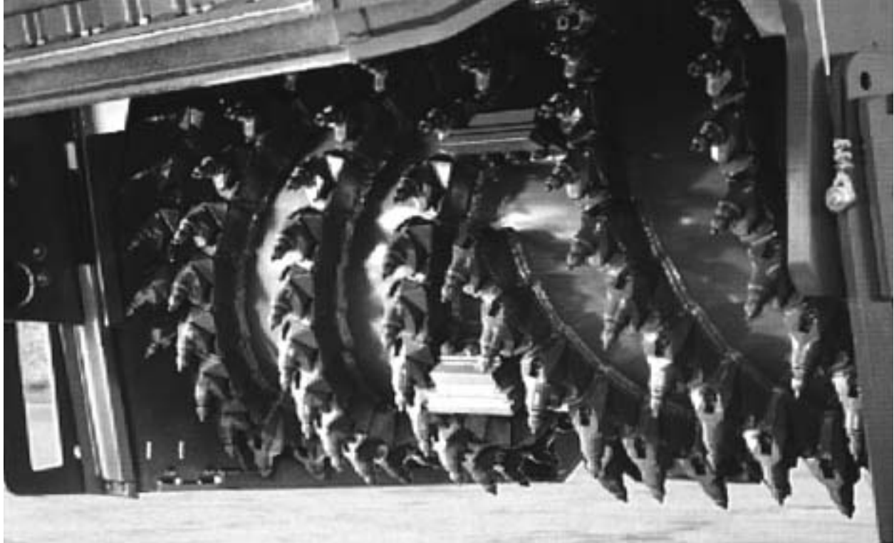
Figure 8-5: Helical pattern of tungsten carbide tools on cutting drum
