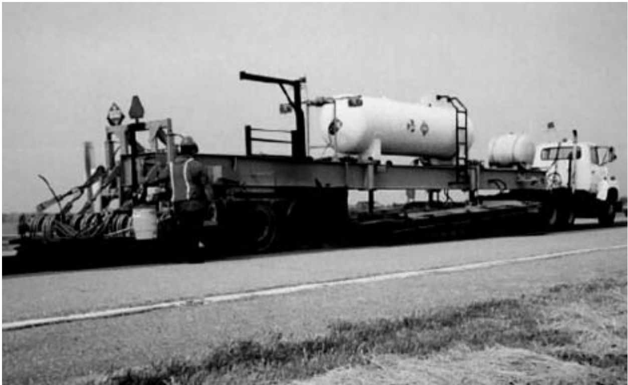
Figure 6-2: Heating and scarifying unit
