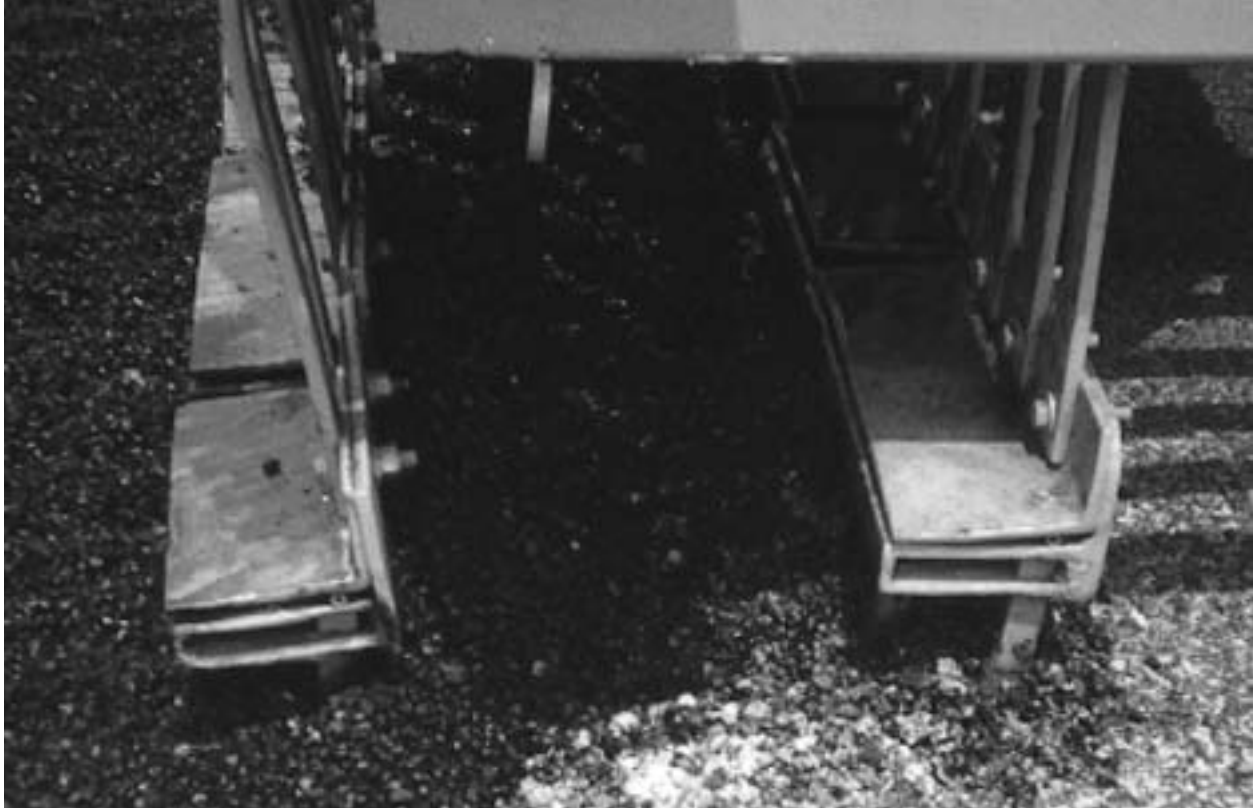
Figure 1-8: Surface Recycling scarification teeth
