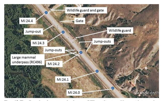
Figure 15: The mile markers, large mammal underpass, wildlife guards, gates and jump-outs between mi marker 24.0-24.4 at the potential concentration of large mammal-vehicle collisions in the Ravalli Curves area. Note that there is a wildlife fence in this area on both sides of the road that ties together the large mammal underpass, the jump-outs, and the wildlife guards and gates.
