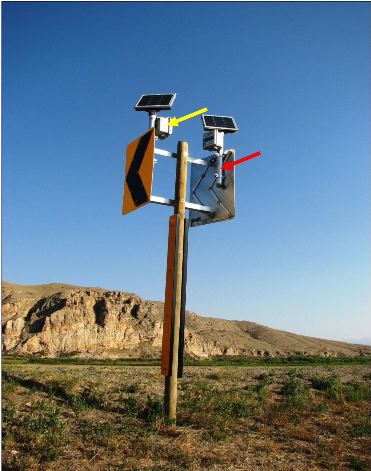
↑ One of the six dual BlinkerChevron's installed on site. The chevron components are fixed on a four (4) inch post with added reflector panels. Each individual LED chevron has its own solar panel and slave radio control unit (yellow arrow). As in the advance signal master control, the NiMH battery is located in the tube bracket (red arrow).
