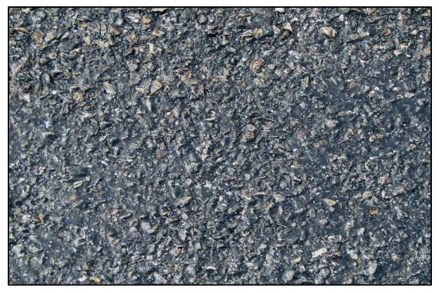
♠ Close-up of average texture of the fog seal over seal and cover (test).
