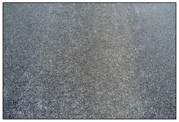
♠ Representative average texture of the fog seal on seal and cover (test).
