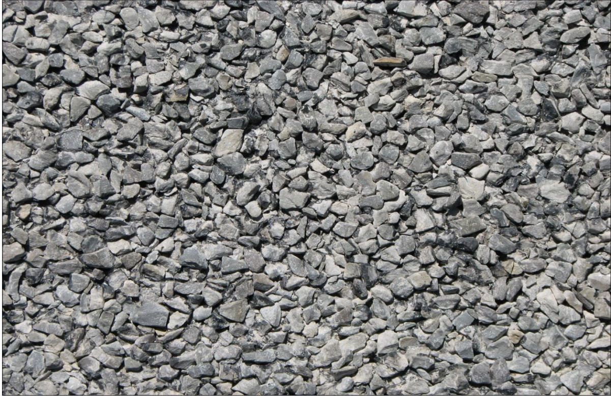
↑↓ Average visual appearance of chip seal embedment on project after cure and sweeping phase completed.
