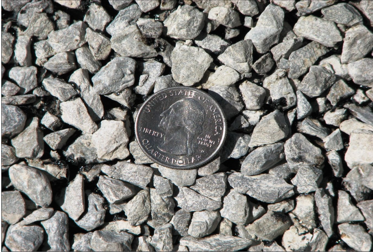
↑↓ Comparison of the level of residual bitumen binder within the Type 2 aggregate to the conventional chip seal and the added fog seal.
