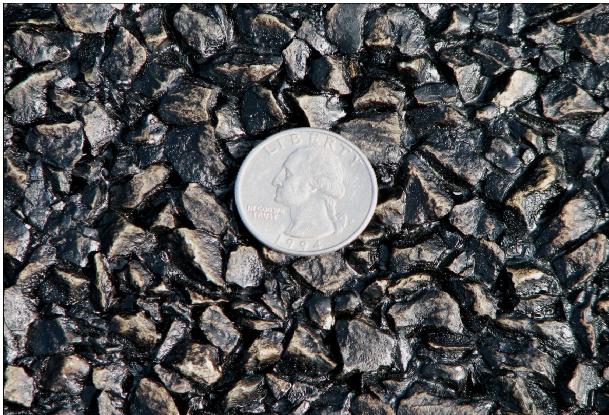
↑↓ Comparison of the level of residual bitumen binder within the Type 2 aggregate to the conventional chip seal and the added fog seal.
